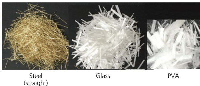
Figure 1.3 Steel, glass and polyvinyl alcohol (PVA) fibres
