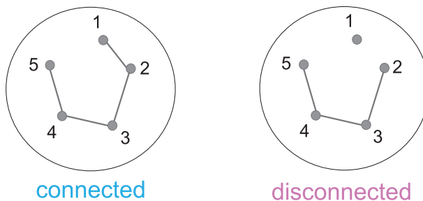
Figure 3.8. Graph connectivity: (Left) An example of a connected graph; (Right) An example of a disconnected graph.
